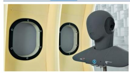
Acoustic test room for airplane primary insulation
