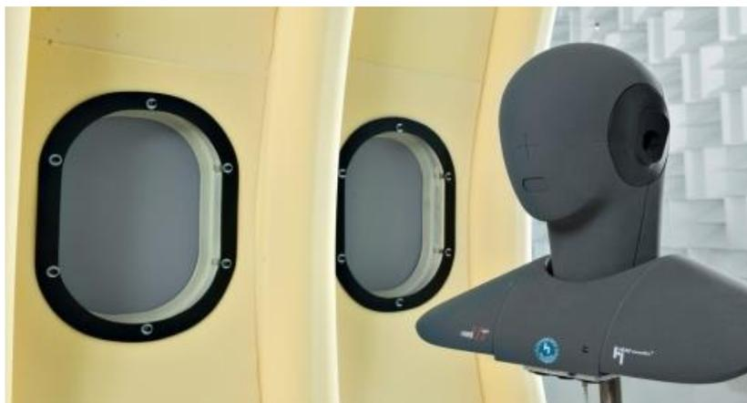
Acoustic test room for airplane primary insulation
