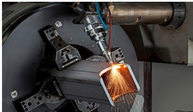
TTM Laser 3D cutting system for profiles and tubes
