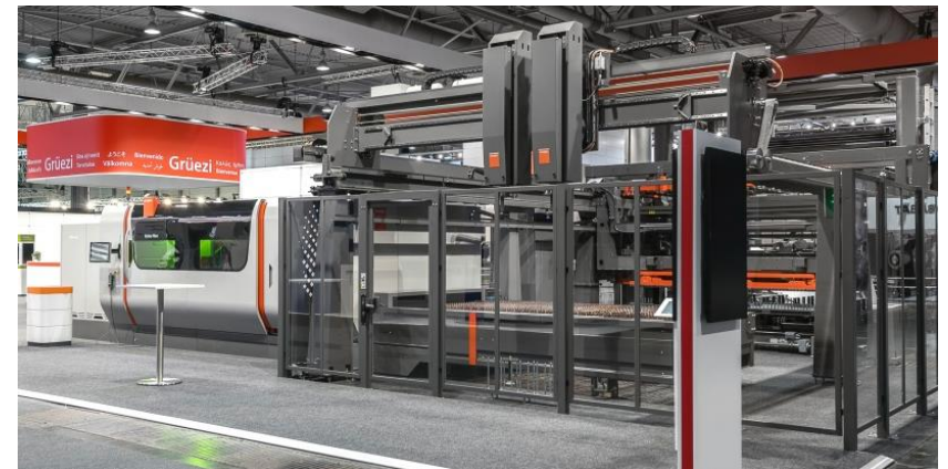
Fully automated production cell: ByStar Fiber with ByTrans Cross and BySort as presented at 2016 EuroBLECH
