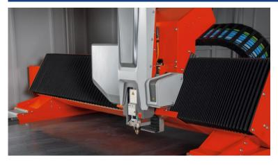
ByStar Fiber flagship product, enhanced with 12 kilowatt laser, new beam shaper function and newly designed cutting head
