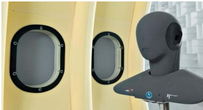
Acoustic test room for airplane primary insulation
