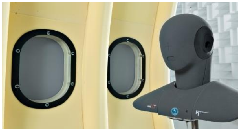
Acoustic test room for airplane primary insulation
